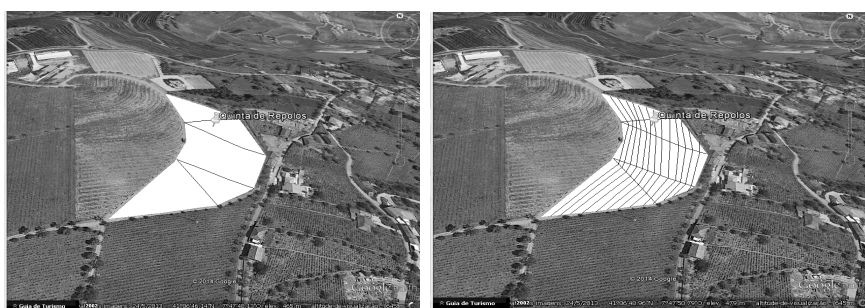
Figure 9 Division of the vineyard into simple geometric figures, for better spatial orientation (left) and scheme of parallel lines for alignment and planting (right)
