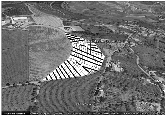
Figure 10 The marking of perpendicular lines (thick line), which are the alignment columns
